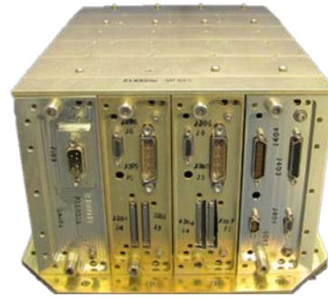
SpaceCube v2.0 Pictured with 1 Power Card, 2 Processor Cards, 1 Digital I/O Card
